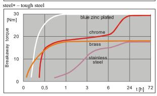
The graph shows the increase in the breaking torque of threaded connection as a function of time at using activator A. The tests were carried out in accordance with to ISO 10964 using M10 bolts and nuts coarse thread.
